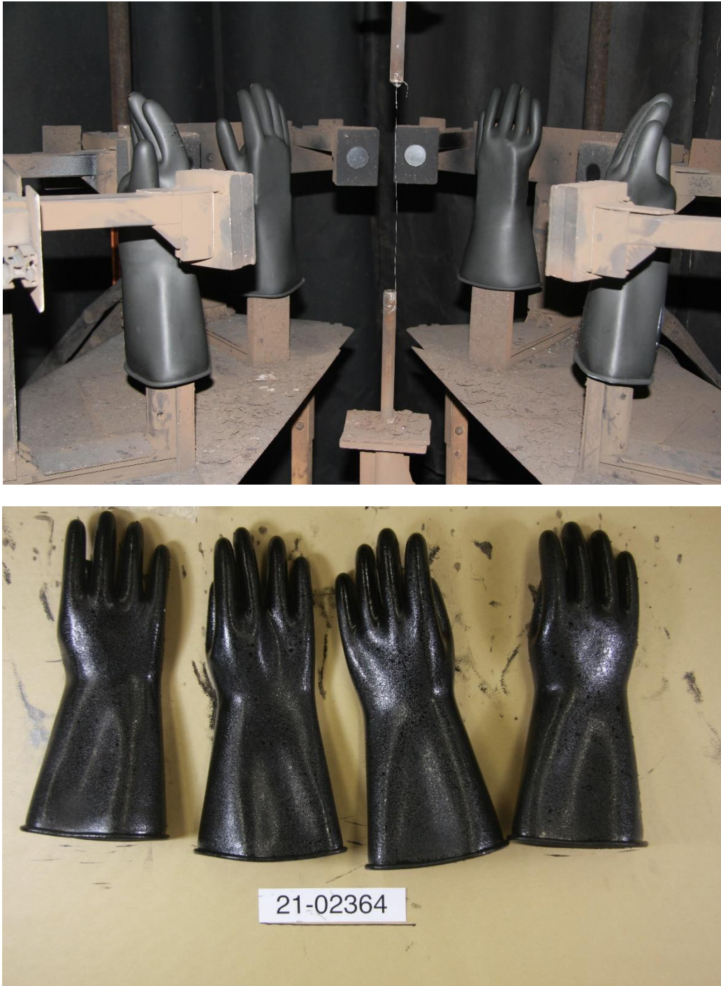
Figure 6-1: Photograph of a specimen before and after arc exposure.
